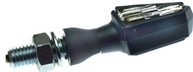
YM-19107ELEDW-1 LED Turn Signal w/Rubber Stem Black Case, and Clear Lens
